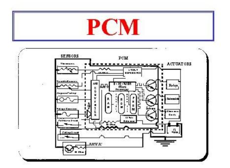
The PCM is the on-board computer which receives input from various sensors and, with this information, controls various engine & emissions control actuators.
