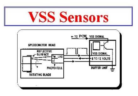
Vehicle speed sensors convert vehicle speed into a digital or analog signal that is sent to the PCM. This information can be used by the PCM for transmission shifting, cruise control, and over-speed control. Vehicle speed sensors can be a Permanent Magnet Generator, a Hall Effect switch, LED photo or a reed switch.
