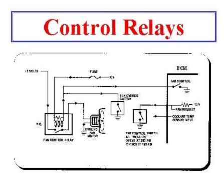
Relays are used to control circuits which require more current than the PCM can handle. The relay uses a low current circuit to control a higher current circuit such as a cooling fan or fuel pump. Relays use an electric magnet to pull high current contacts together or apart, depending on the application.
