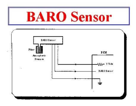
A BARO sensor is basically the same as a MAP sensor but is used to monitor barometric pressure only. In many cases the MAP sensor will take a reading of the barometric pressure as the engine is started. This reading is usually stored by the PCM until the key is turned off. Some systems will update the Baro reading during certain driving conditions. When testing an intermittent problem try lightly tapping on the sensor to show up the fault.
