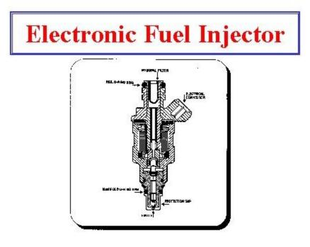
Fuel injectors are a Solenoid used to deliver fuel and are pulsed on to control the air fuel mixture. Injectors are usually energized for 1.5 to 3 milliseconds at idle. An on time of more than 5 MS usually indicates a rich command.
