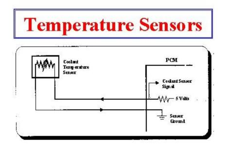
These types of sensors are called a "thermistor". This simply means that as the temperature changes the voltage signal changes. Most thermistor type sensors are of the NTC type. NTC means "negative temperature coefficient". This means that as the temperature of the sensor increases, the electrical resistance decreases. There are a "few" PTC type temperature sensors which increase in electrical resistance as the temperature of the sensor increases.
