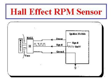
RPM sensors convert engine RPM into a voltage signal which the PCM uses for RPM, ignition timing, injector timing and over rev control. RPM sensors are also used to trigger the module when controlling the primary ignition.
