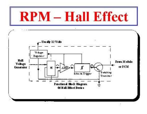
RPM sensors convert engine RPM into a voltage signal which the ECM uses for RPM, ignition timing, injector timing and over rev control. RPM sensors are also used to trigger the module when controlling the primary ignition.
