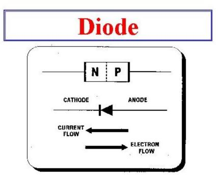
Diodes are a semiconductor designed to allow current flow in one direction only. Some vehicle manufactures use diodes within some circuits to restrict current flow to one direction only. Diodes also are used across some solenoids and relays to protect the PCM from inductive voltage spikes. Some motors, such as cooling fan motor, have diodes in them to reduce the A/C voltage that is produced within the motor.
