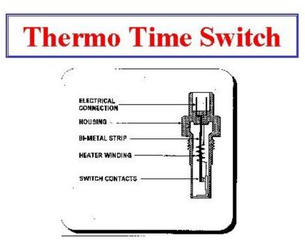
Some manufactures use a cold start injector to enrich the air fuel mixture during cold start-ups. These injectors are not controlled by the PCM. They use a thermo-time switch to complete the ground circuit for the cold start injector.
