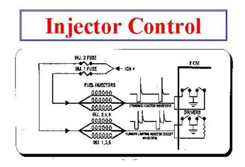
Fuel injectors are a Solenoid used to deliver fuel and are pulsed on to control the air fuel mixture. Injectors are usually energized for 1.5 to 3 milliseconds at idle. An on time of more than 5 MS usually indicates a rich command. The injector has two wires, usually one supplies system voltage (key on) to the injector and the circuit is completed (grounded) through the other wire via the PCM.
