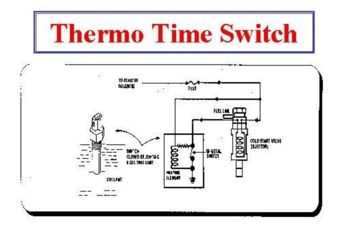
Some manufactures use a cold start injector to enrich the air fuel mixture during cold start-ups. These injectors are not controlled by the PCM. They use a thermo-time switch to complete the ground circuit for the cold start injector.
