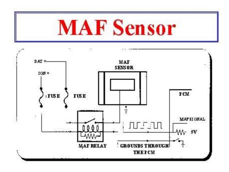
MAF sensors convert the intake air flow and air mass into an electrical signal. This information can be used by the PCM for fuel delivery and spark timing. MAF sensors will send either a digital or an analog signal depending on the type and the manufacture. Most sensors use a hot wire or a heated element to measure the air flow. As the air flows past the heated element (or wire) the element is cooled. This cooling changes the resistance, and thus, the current flow in the element.
